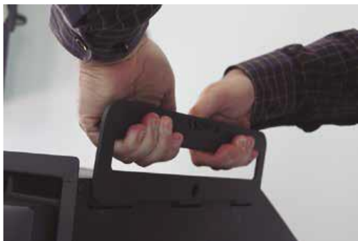
Figure No.3 - Positioning the handles for transferral
